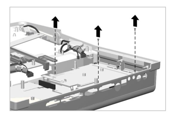
Figure 6-19. Removing the MultiBay Assembly Screws
